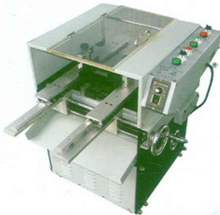
Automatic Lead Cutting Machine
